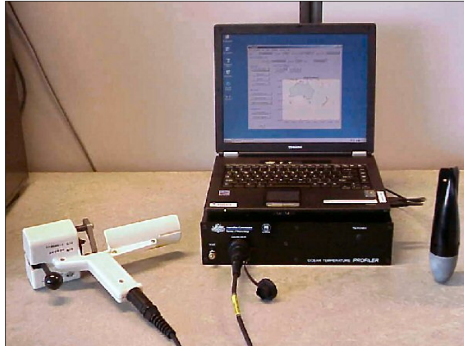
Devil XBT System as used by the Australian Bureau of Meteorology
