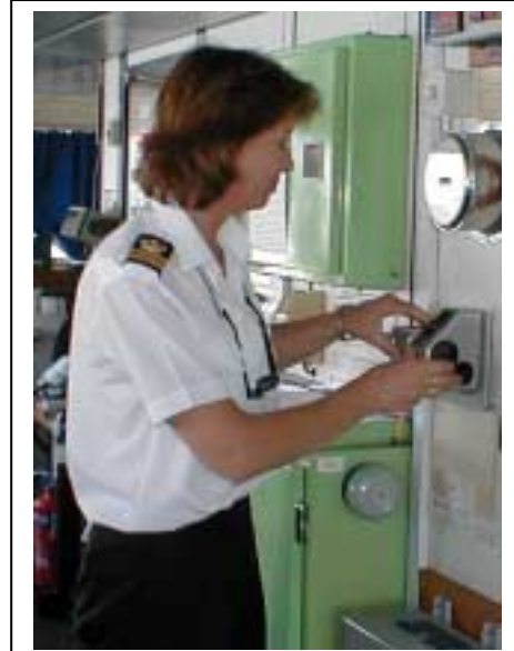
Observer Suzanne Allen 2/O checking the pressure using a Precision Aneroid Barometer on the RRS Charles Darwin [Photo by H. Gale. PMO]
