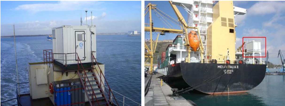
Figure 1 : 10ft container launchers on board the ATLANTIC COMPANION and MELFI ITALIA II.
