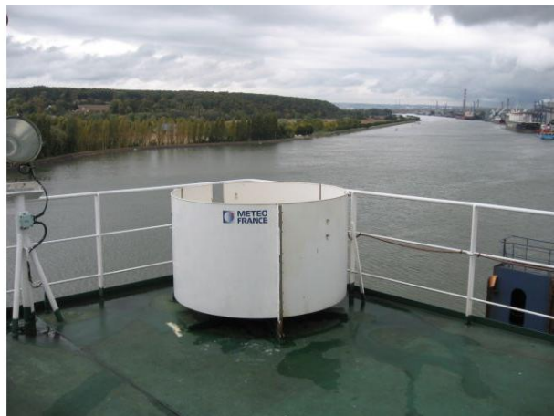
Figure 2 : Installation of open deck launcher on board a French ASAP ship.
