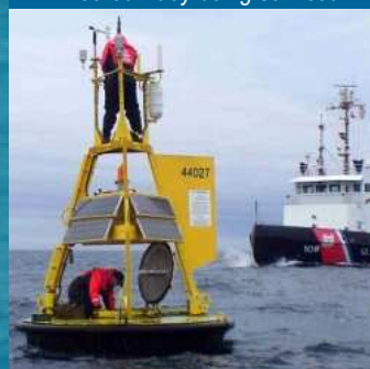
A Moored Buoy being serviced
