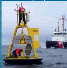
A Moored Buoy being serviced
